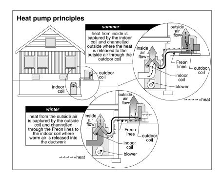
As with conventional air conditioning, the compressor is the most critical component.
