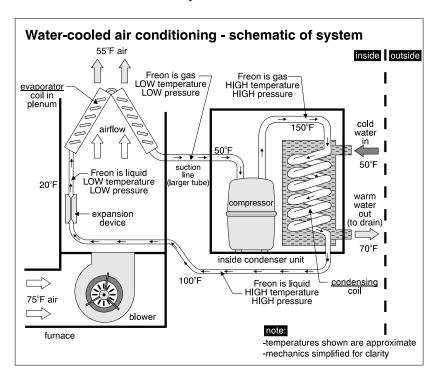
Once the water has cooled the gas back down to a liquid, the warmed water must be disposed of. It is no longer drinkable and, therefore, must go down the drain. As an alternative, some people use the warm waste water to fill a swimming pool or water the lawn.
