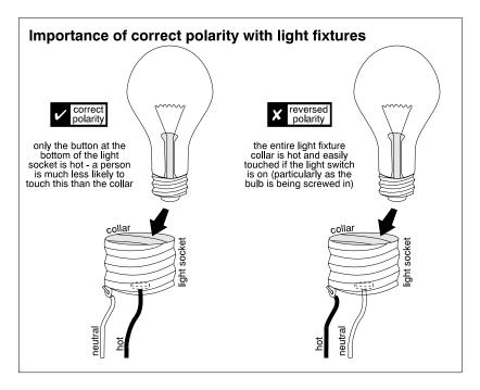
Corrective action simply involves disconnecting the circuit and re-connecting the wires, so that black joins brass and white joins silver.
