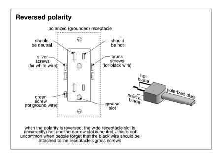
A reversed polarity outlet can compromise the safety of an electric appliance, depending on how it is wired. A grounded appliance may have its grounding made ineffective by reversed polarity.
