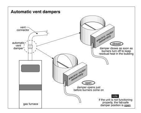
improves the seasonal efficiency. These systems are designed to be fail-safe. In the event the vent damper does not open, the furnace or boiler will not come on (if it did come on, all of the exhaust gases would end up in the house).
