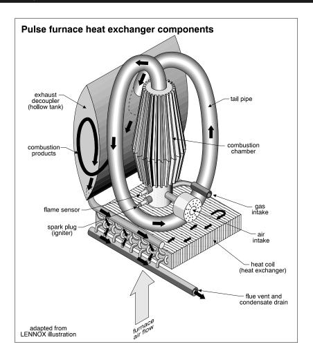
Since there are more components in a high efficiency system, there is more to go wrong and, consequently, regular maintenance should be somewhat higher than a conventional furnace. At least annual servicing is required.
