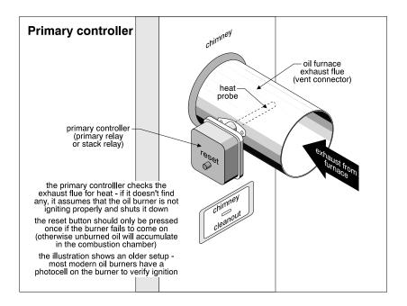
be pressed only once if the furnace fails to ignite. Pushing the reset button several times could allow an unsafe accumulation of oil in the combustion chamber. Some newer oil burners use a cadmium sulfide "eye", or photocell, on the oil burner that verifies ignition.
