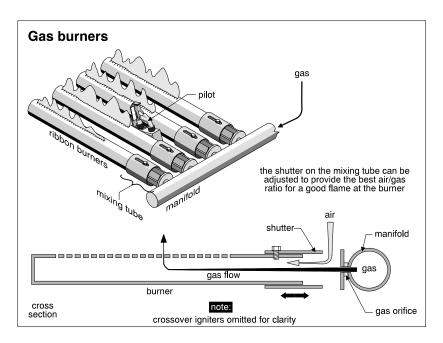
A gas burner is fed from a valve which allows gas to enter the burner where it is mixed with air and ignited. Gas burners can be of several shapes; however, the most common type is the ribbon burner which is not unlike the burner found on a gas barbecue.
