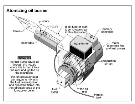
An oil burner is somewhat different since it is dealing with a liquid fuel rather than a gas. A pump is used to force the liquid fuel through a nozzle, causing it to atomize (break up into small droplets). A fan blows air through the burner to mix with the atomized oil. The mixture is ignited by a spark, creating combustion.
