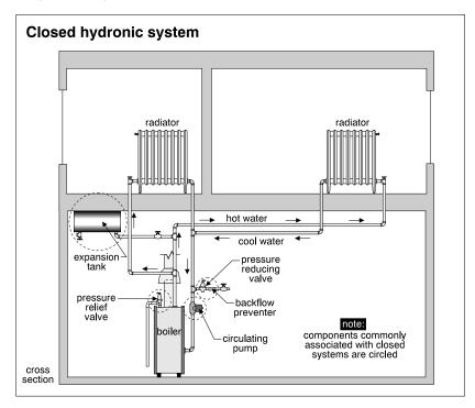
Closed Systems Modern boilers are "closed" systems. The water in the boiler, in the piping, and in the heat source within each room, is under pressure. The pressure within the system is normally a few pounds higher than what is required to force water up to the highest level within the house. In a typical house, this pressure would be twelve to fifteen pounds per square inch.
