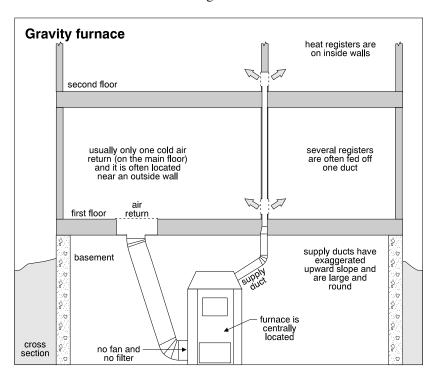
Almost all gravity warm air furnaces are obsolete and even if the heat exchanger has not failed (which would require immediate replacement of the furnace) a good argument can be made for replacing the unit because of the inefficiency of the system. Reduced heating costs would pay for a new furnace in a few years.
