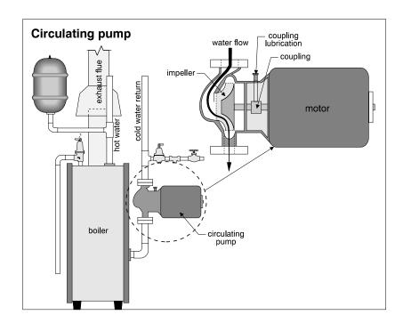
Many modern boilers (e.g. copper tube boilers) have a safety interlock that prevents the boiler from operating unless the pump is running. These boilers would quickly overheat if water was not flowing through them.
