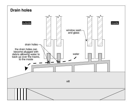
Problems include low quality hardware subject to breakage, tracks at the bottom which don't drain water to the outside, poorly fit slides, and poor joints at comers of the frames. Leaks often result in water damage to wall finishes below the windows, most often at comers. Exterior caulking may help in some cases; in others, storm windows added on the outside improve weathertightness. Where the problem is chronic, replacement windows may be the best answer.
