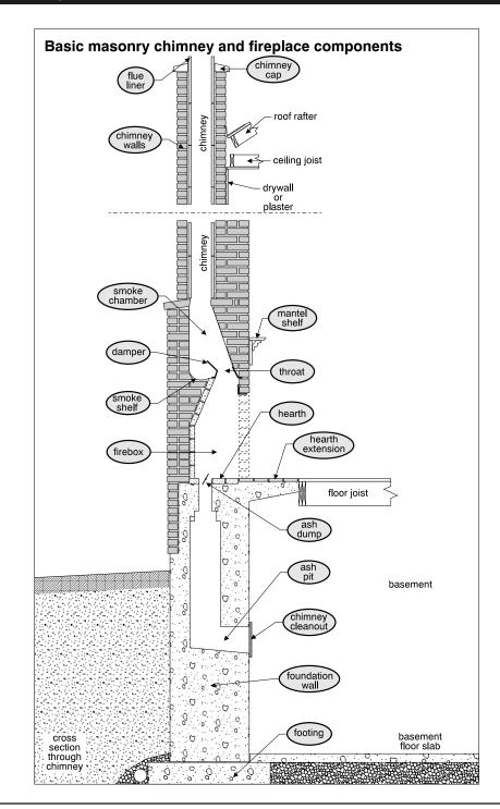
**8.1.1** Ash Dumps: Some fireplaces have a trap door in the hearth to allow cool ashes to be dumped into a pit below the fireplace. The ash pit can be emptied from below. This eliminates the need to sweep ashes into a container and carry them through the house. Ash pits should be separated from combustibles by at least four inches of solid masonry. Missing ash dump doors in fireplace hearths should be replaced prior to using the fireplace.
