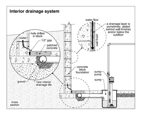
This approach is somewhat less desirable than the exterior approach, since water has no natural inclination to find this drainage tile. Water may accumulate on the outside of the foundations for some time and may leak through the exterior walls before it is carried away by this drainage system on the inside. The water, of course, must pass through the foundation or footing system, or go under the footing to reach this tile. In rare cases, this can undermine the footings.
