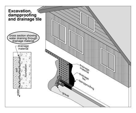
In modern construction, the piping used is perforated plastic, and it is arranged to discharge straight into a storm sewer. The perforated plastic piping which has replaced the clay tile piping is corrugated and very flexible. The perforations are in half of the diameter of the pipe only. The piping should be laid with the holes down.
