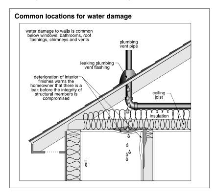
Roof leaks are usually localized and the source of the problem will often be an intersection or a flashing in the roof. Roof leaks can be difficult to trace because the water does not always appear on the interior immediately below the leak above. This may be the result of water running along framing members, or vapor barriers which prevent water coming through in specific locations. Many roof leaks appear first around ceiling light fixtures, for example.
