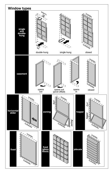
Some modern high quality double hung windows are pivoted at the bottom, and when release pins at the top are moved, the window can be rotated out of its normal operating plane, into the room so that the outside of the glass can be easily cleaned without going outdoors.
