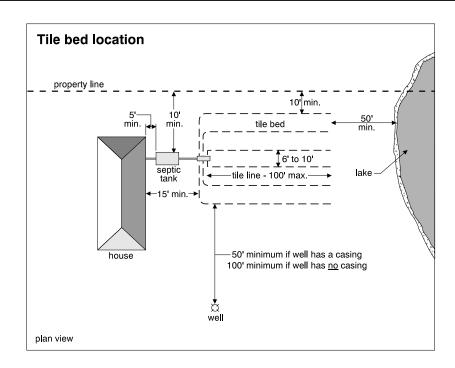
Problems which lead to failure of septic systems include overloading of the tile bed, soil breakdown around the tiles, high water tables, clogging of the tiles, and broken or cracked tanks and tiles.
