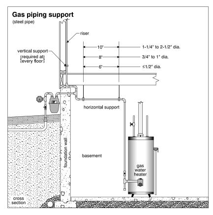
Appliance Connections Where appliances are connected, there should be a shut off valve in the same room for each appliance, as close to the appliance as is practical. Unions or swing joints should not be in concealed areas (walls, attic, et cetera).
