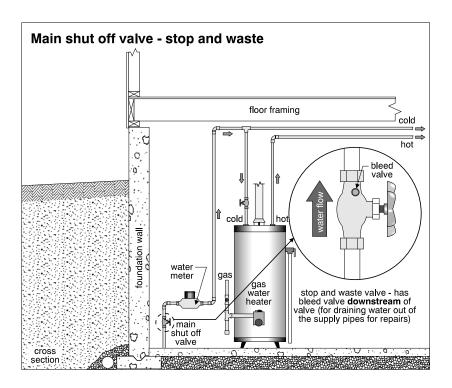
Partly Closed Poor house water pressure is occasionally the result of partially closed main valves. This, of course, is easily corrected.
