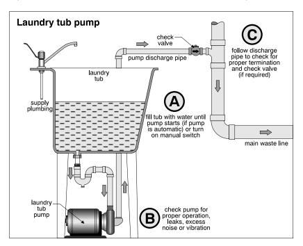
Some pumps have an automatic control (typically a float system within the tub), although many are manually operated by a wall switch. The laundry tub is typically large enough to hold the water from a complete cycle of a washing machine. When the washing machine cycle is completed, the pump is turned on briefly to drain the laundry tub. Either arrangement is satisfactory.
