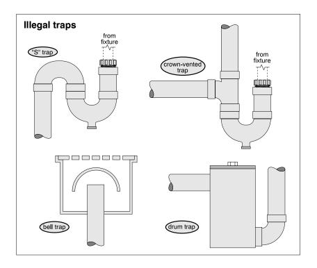
Most fixtures require traps, although a toilet does not, since the water in the toilet bowl creates a natural trap. Dishwashers are usually effectively trapped, although there is no formal fitting. The drain line from the dishwasher should be arranged to form a trap.
