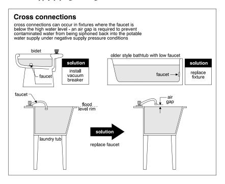
The obvious solution is to raise the faucet set above the top of a tub or basin. This is common practice in modern plumbing, and cross connections do not occur under normal circumstances. Cross connections are also avoided through the use of an overflow. In bathtubs, for example, where the faucets may enter through the wall of the tub below the top, an overflow provided below the faucets will prevent a cross connection.
