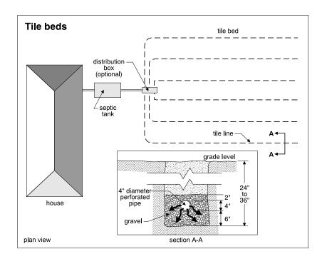
Special sand can be used which allows very small tile beds to be installed. This is expensive, since the sand has to be brought onto the site, but it may be important to keep the tile bed small. These special tile beds are used with conventional septic tanks, or can be used with the mechanically assisted systems described above.
