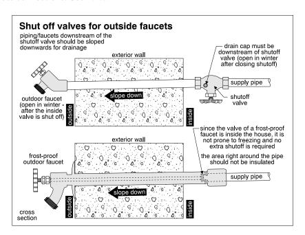
There are special frost-proof outside valves which have long stems going through the wall, to shut off the water inside the building every time the faucet is used. These frost-proof valves do not require permanent shut off in the winter. Hoses must be disconnected and the values must be sloped to allow the valves to drain and prevent freezing.
