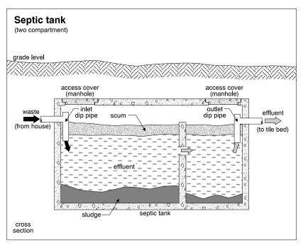
Most of the material which enters the tank is in a liquid state. Within the tank, the majority of the solids are broken down to gases and/or liquids. The breakdown takes place as a result of bacteria action, both aerobic and anaerobic. The liquids are discharged from the tank into the tile bed. The gas escapes through the plumbing vents.
