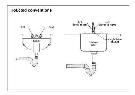
**3.2 Basins** (Lavatories): Basins, typically located in washrooms or bathrooms, may be made of stainless steel, enameled steel, enameled cast iron, copper, vitreous china, plastic, marble, simulated marble, etc. None of these materials will last forever, and all have their strengths and weaknesses.
