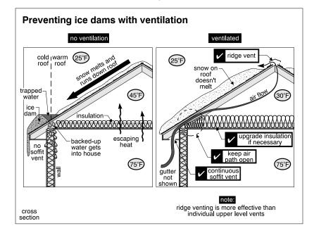
Ice dams are most common on low slope roofs or roofs which change from a high slope to a low slope. The largest dams tend to form over unheated areas, such as eaves, porches, and attached garages. Ice dams are also common above party walls in attached houses.
