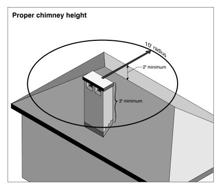
The best solution is to extend the chimney upwards. Alternative solutions such as a wind cap or adding glass doors on a fireplace are effective in some cases.
