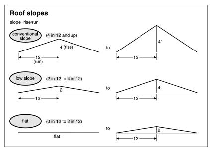
Roofs with a pitch greater than four in twelve are considered conventional roof systems. Roofs with a slope between four in twelve and two in twelve are considered to be low slope roofs, and roofs with a pitch less than two in twelve are considered to be flat roofs.
