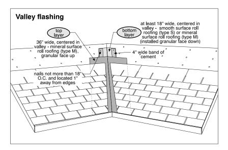
*Problems* Valleys are particularly weak spots on roofs, as they channel a significant amount of water; therefore, even a small leak can cause considerable damage. The slope of the valley is less than the slope on either side. This causes increased wear on the valley. Sometimes valley flashings stop short of the edge of the roof and allow water to pour into the eaves. Also, the inexperienced tend to walk up valleys when traversing a roof. This damages valley flashings,
